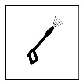
When this power wash icon is displayed, this means the fixture is rated IP69K.
